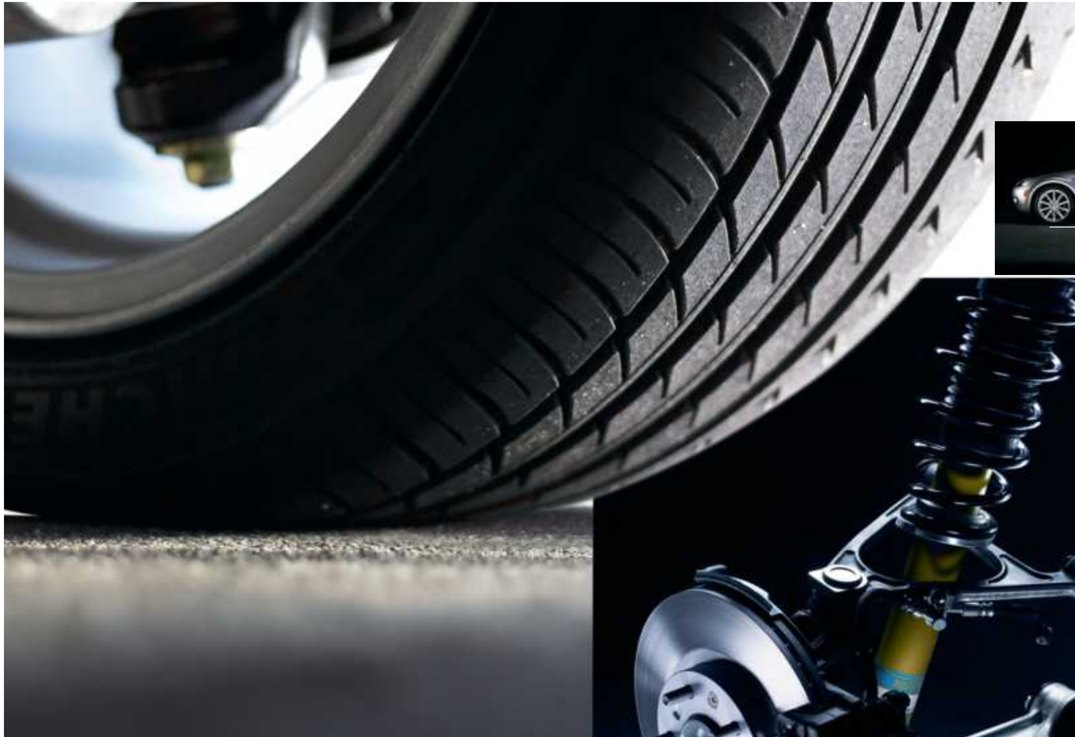
A. The MX-5 Miata's hollow front stabilizer bar helps reduce weight and minimize body roll while helping to maintain tire contact—especially during abrupt directional changes. B. An advanced double-wishbone front suspension, featuring aluminum alloy control arms and gas-filled shocks, helps promote quick response to all driver input and contributes to the MX-5 Miata's superb handling. Power-assisted ventilated front disc brakes with large 11.4-inch rotors promote consistently linear, fade-resistant stops.
